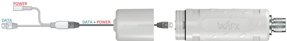
PoE Ethernet port supports 10-48VDC through the injector. Alternatively, it can be powered through the USB-C connector for service and initial configuration.
